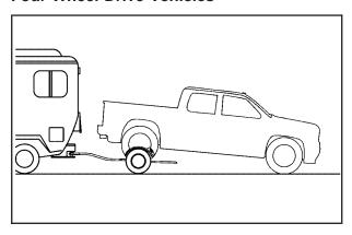
Use the following procedure to dolly tow a four-wheel-drive vehicle from the rear:
